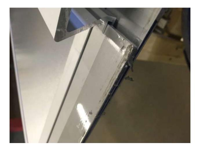
The wheels on panel #4 had significant black powdery residue around them where this was not present on any others. It is inconclusive where this is coming from but it may be a result of some late stage drilling operations during set up that allowed for some aluminum drilling residue to be present near the end of the track for panel #4.
