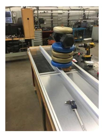
Deflection on the acrylic portion of the panel was 0.458in and on the aluminum outer edge it was 0.347in. Load was applied on a 4in x 4in wooden puck eccentrically.
