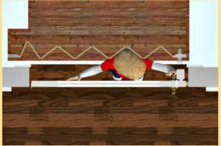
Figure 9: Representation of child trapped between door and accordion carriage gate; graphic courtesy of Fair Warning
