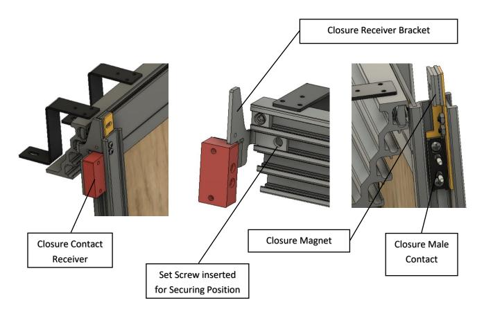
The above shows the standard contact switch that is supplied and should be installed as part of the gate set up.
