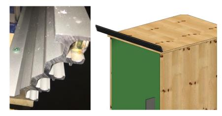
The support method is designed for 3/4in plywood support or equivalent. If you are using other materials that could have tear out concerns (melamine/ MDF) you should consider adding additional screws by simply drilling additional holes in the tail of the upper track where the others are located and it may also need to use appropriate screw anchor inserts.
