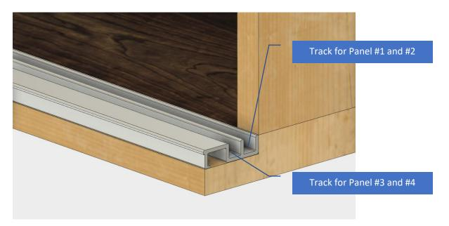
Push panel #1 to the back of the channel such that the lower aluminum cross piece is touching the surface of the track that is furthest from the landing side.
